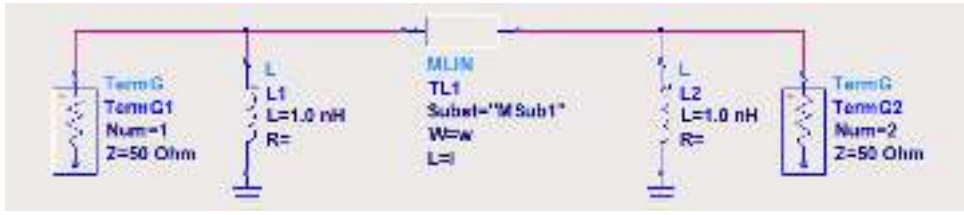
Figure 55: DUT - line with length L , 50\Omega and shunt inductance equal 1nH .
