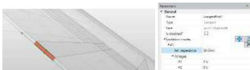
Figure 6: The idea of the definition lumped port on the side wall. In this case it is small rectangular area between the strip with conductor and the groundplane.
