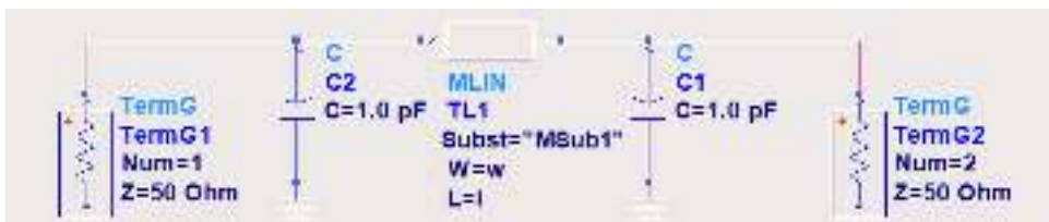
Figure 27: DUT - line with length L , 50\Omega and shunt capacity equal 1pF .
