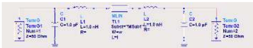
Figure 70: DUT - line with length L , 50\Omega and series inductance equal 1\text{nH} and shunt capacity equal 1\text{pF} .
