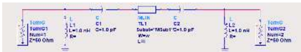
Figure 32: DUT - line with length L , 50\Omega and shunt inductance equal 1\text{nH} and series capacity equal 1\text{pF} .
