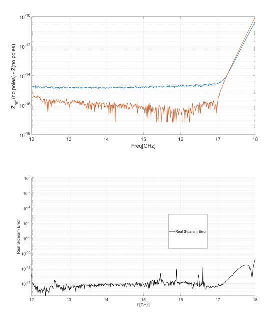
• for the projection basis composed of all the eigenvectors and 12 block moments (24 vectors). The whole projection basis contains **41 vectors** (17 + 24).
